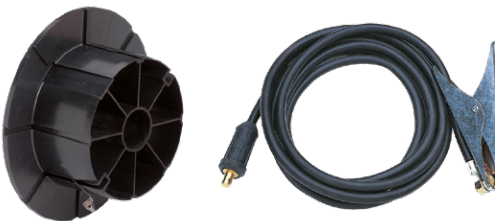
Work return cable and basket spool adapter Work return cable and plug 25 mm², 4 m long, plug 13 mm. Adapter for insertion of a welding wire basket spool.
