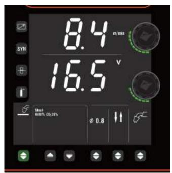
Once the machine has been setup for MIG (as above along with page 30) you will be in a position to setup the control panel for your MIG welding task.
