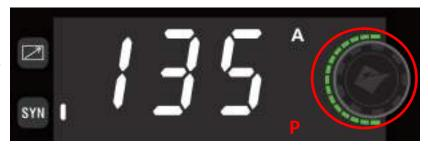
operator through amperage control, wire feed speed and material thickness as shown below:
