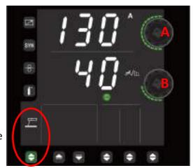
Please Note: Welding current adjustment can be carried out during welding.
