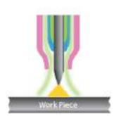
The main challenge with scratch start TIG welding is keeping your electrode clean. While a quick strike with the electrode on the metal is essential and then not lifting it more than 3mm away to create the arc will help, you also need to ensure your metal is completely clean.
