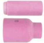
Gas cups are made of various types of heat resistant materials in different shapes, diameters and lengths. The cups are either screwed onto the collet body or gas lens body or in some cases pushed in place. Cups can be made of ceramic, metal, metal-jacketed ceramic, glass or other materials. The ceramic type is quite easily broken so take care when putting the torch down.
