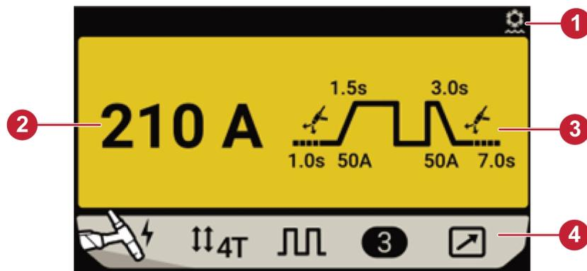
1. Water cooler connection: water cooling symbol is display in status bar when water cooler is connected and activated.
