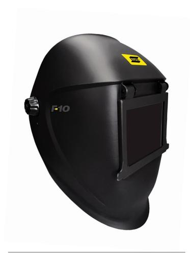
F10 (formerly Eco Arc II) has a 'flip up' front in to which a welding glass is fitted. There is also a protective plastic lens that gives facial protection when the front is in the up position. F10 is available in three flip front options, the helmet also adopts the Eco Head Gear, with 5 rake positions.
