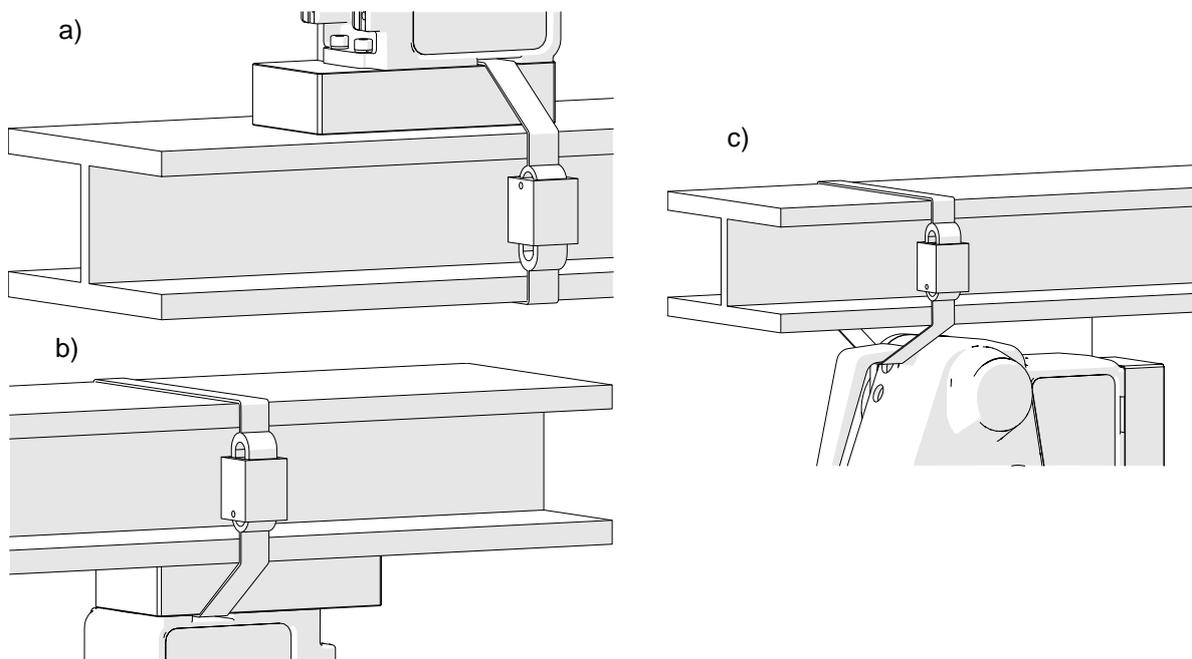
**Figure 7.** Securing the drilling machine using the safety strap
