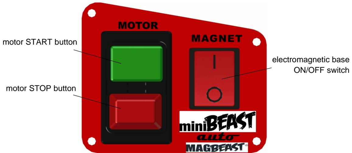
**Figure 2.** Control panel design
