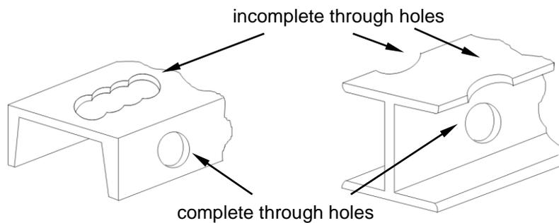
**Figure 5.** Types of holes to establish with annular cutters
