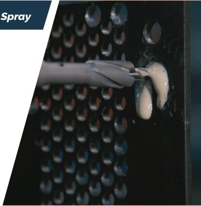
SpeedLube™ is a high performance foaming lubricant suitable for a wide variety of metal drilling applications across a range of materials including stainless steel.
