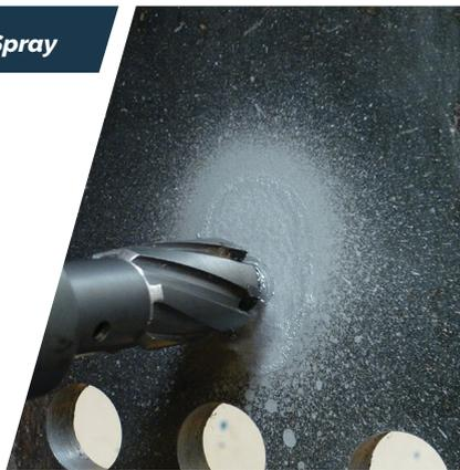
AeroPaste™ is an aerosol applied paste-type, metalworking lubricant for hole broaching, tapping, reaming & drilling applications. Ideal for overhead or positional application, the high viscosity of AeroPaste allows it to cling directly to the cutting tool or steel it is applied to, without fluid run-off.
